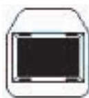
Figure 6-7: USB X7, USB-B-S-S-B-TH (4 pins).
