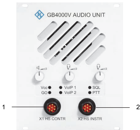
Figure 2-6: External interface, front view R&S GB4000V (VAR03).
